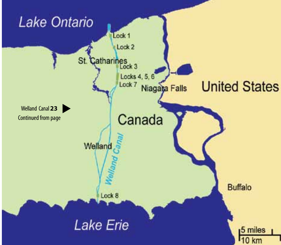
▲ This map of the Welland Canal shows the location of the eight locks needed to sail between Lakes Erie and Ontario, which is at a much lower elevation. Note the closeness of Locks 4, 5, 6 and 7 at the Niagara Escarpment. Niagara Falls, which goes over the Escarpment, is the reason that the Niagara River needs to be bypassed. Map by Agyle courtesy of Wikimedia Commons.
